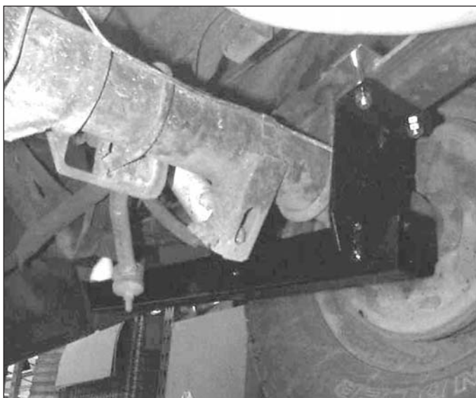
Rear bracket with mounting clamp on top of spring.
