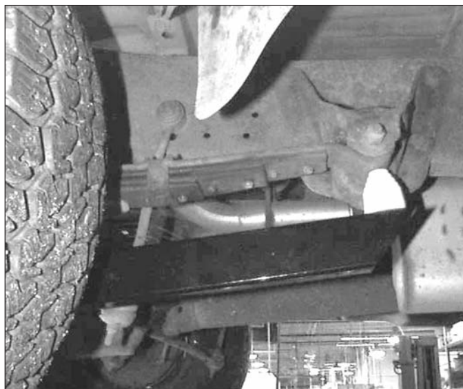
Locate snubber under front spring eye.
