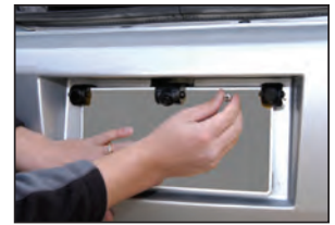
Secure license plate bracket with provided screws
