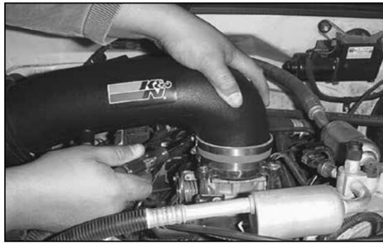
29. On models with air injection, attach the air injection hose to the flange on the vent filter using the O.E. clamp.
