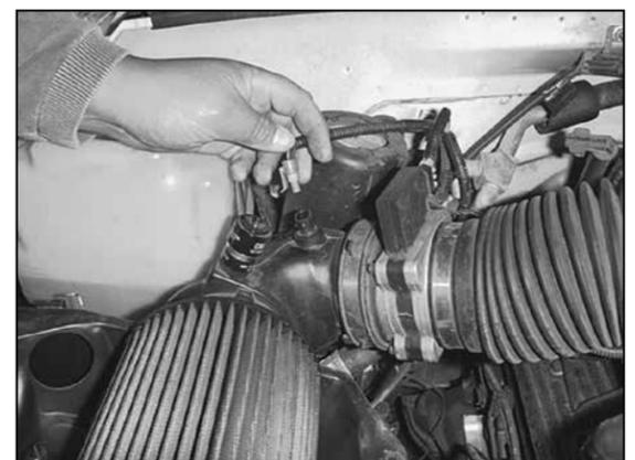
5. Disconnect the air temperature sensor electrical connection.
