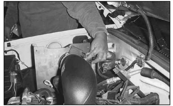
33. Reconnect the mass air sensor electrical connection.
