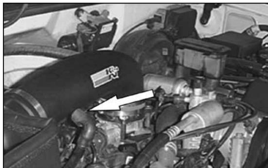
31. Reconnect the crankcase vent hose onto the intake tube.
