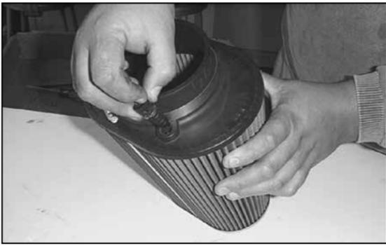
24. Reinstall the factory air temperature sensor into the provided hole on Filtercharger element.
