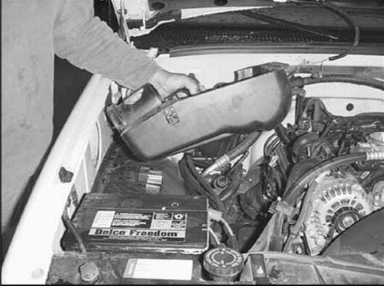
8. Remove the lower airbox assembly.
