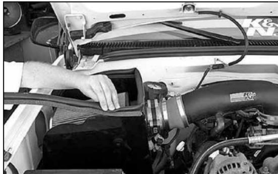
32. Install trim seal onto the heat shield.
