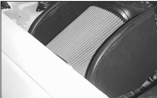
26. Place the filtercharger element into the heat shield and reconnect the air temperature sensor electrical connection, then slide the element onto adapter and tighten with provided hose clamp.
