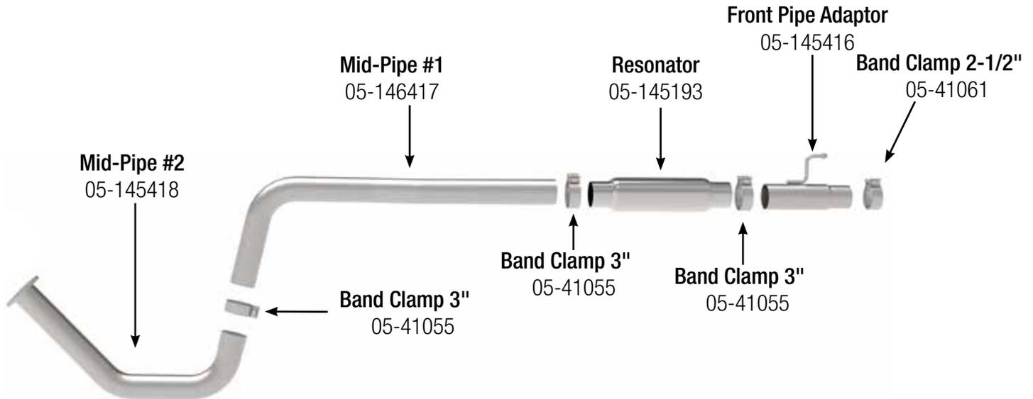
Professional installation is highly recommended. (Read instructions prior to installation). Make sure to always have at least (2) stands or jacks on hand to support the removal of OE system. Also for the installation of aFe system. Any Removal of rubber isolation mounts may require using a spray lubricant such as WD40 and a pry bar.
