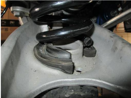
3. Using a screw, or floor jack, raise the lower control arm into position, and align the to the upright. Using a 21 mm socket, and open wrench, torque bolts to 56 ft-lbs
