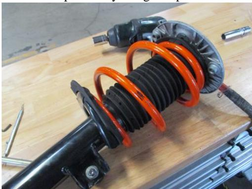
2. Install the strut assembly into the vehicle by lifting into place, and positioning the upper mount to the body. Note there are positioning pins to pilot into the body. Having a helper on hand, reinstall the (3) upper bolts using a 18 mm socket. Torque to 25 lb-ft.
