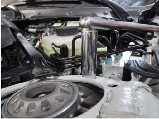
8. Using a strut compressor, remove the factory springs from the strut, by removing the top nut, using a 18mm 12 point socket.
