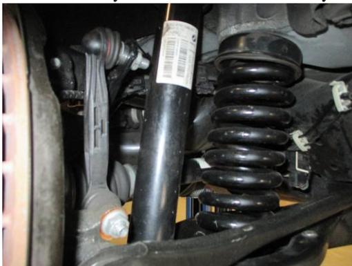
4. Disconnect the ride height sensor located on the driver's side lower rear control arm.
