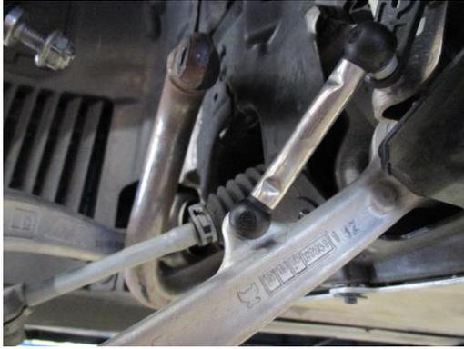
4. Position a screw, or floor jack under the front control arm to hold in place.
