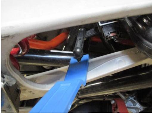
5. Using either a floor jack, or a screw jack, support the lower control arm.
