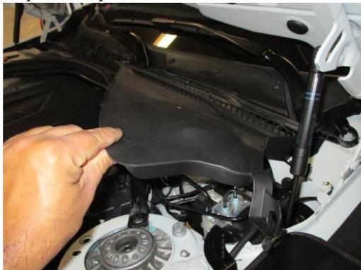
7. Using a 16 mm socket, remove the (3) bolts that hold the strut housing into the vehicle. Be careful to use a helper to hold the strut from the bottom of the car.
