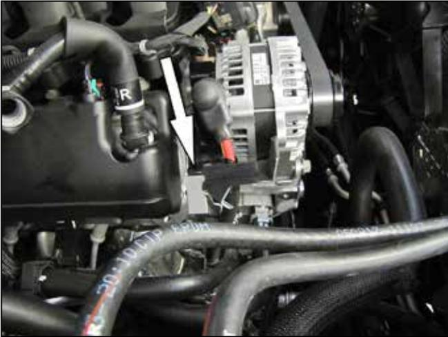
3. On vehicles equipped with the intake plenum support bracket, install the provided spacer between the bracket and cylinder head and secure with the provided hardware.
