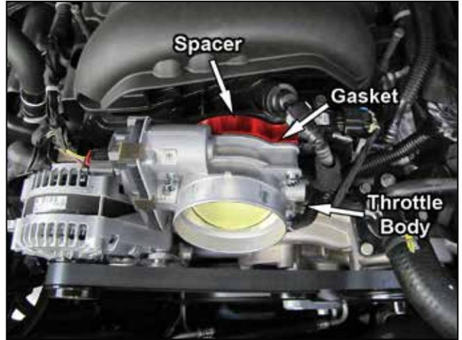
5. Install the provided new bolts through the holes in the throttle body, through the holes in the provided gasket and through the POWERAID spacer. Start the new bolts into the inserts in the intake manifold being careful not to cross thread the bolts. Tighten the bolts in a cross pattern to the factory specifications.
