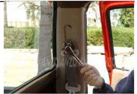
Use the 14mm socket to remove the bolt holding in the seat belt.
