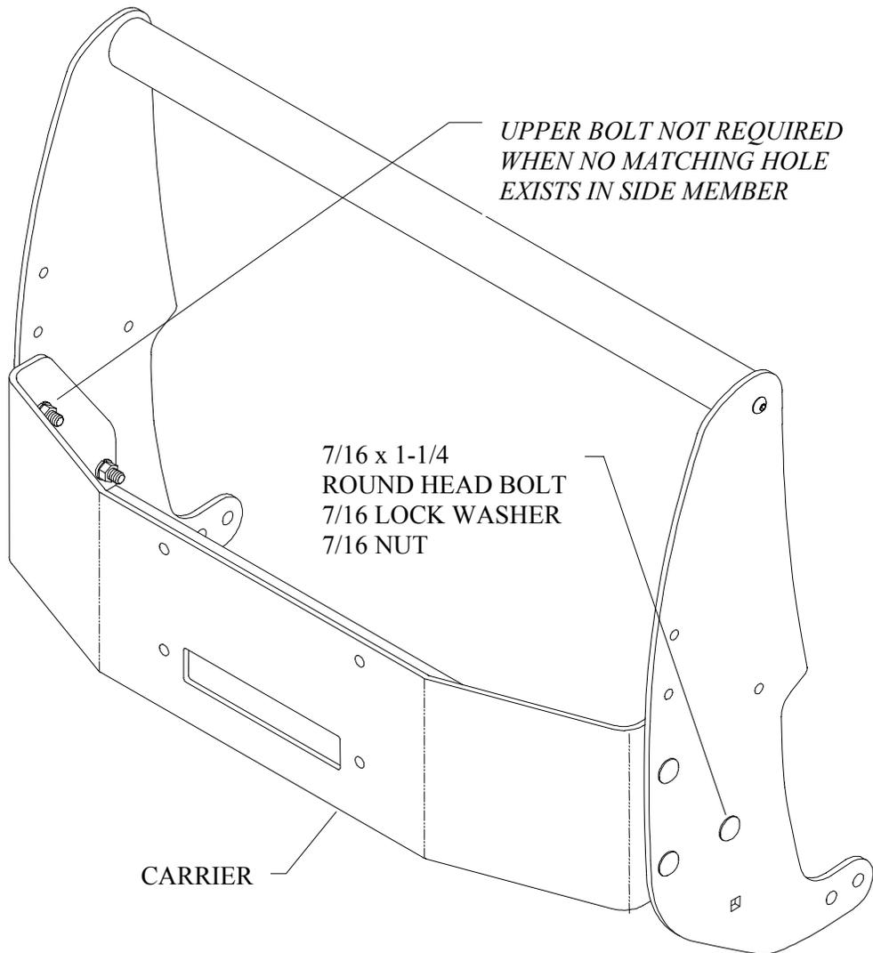
2. If a front license plate is required in your state, it can be attached at the holes provided in the lower stiffener plate of the Carrier.
