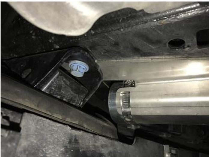
19. Place the reservoir in the bracket and tighten the hose clamps. Hose clamps should be placed through the openings in the bracket.
