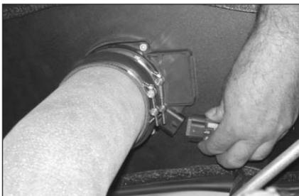
23. Reconnect the mass air electrical connection as shown.
