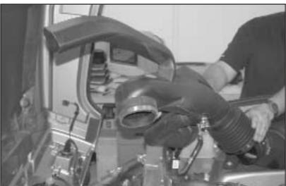
6. Detach the intake tube from the throttle body and mass air sensor then remove the intake assembly. NOTE: K&N recommends that customers do not discard factory air intake.
