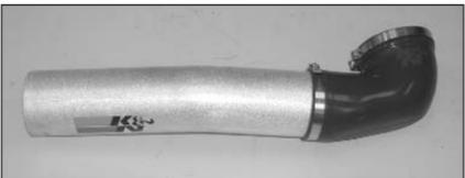
19. Install the silicone hose (084053) onto the K&N intake tube as shown using the supplied hose clamps.
