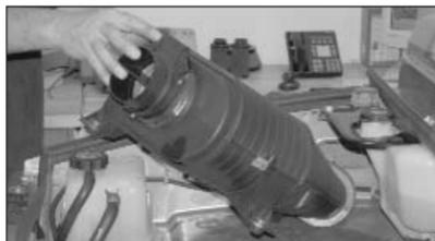
8. Remove the air box from vehicle as shown.
