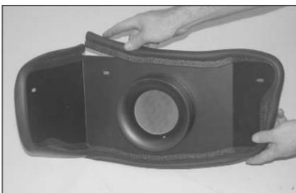
11. Install the edge trim onto the heat shield. Trim if needed.
