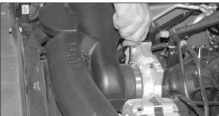
4. Loosen the hose clamp at the throttle body.
