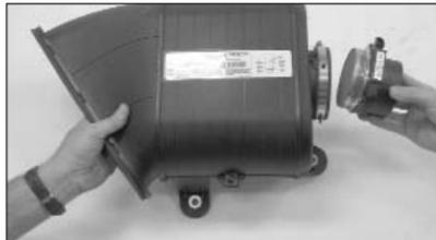
9. Loosen the hose clamp that retains the mass air sensor onto the air box then remove the mass air sensor from the air box.
