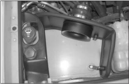
18. Secure the brackets to the heat shield with the provided hardware. Do not tighten completely.
