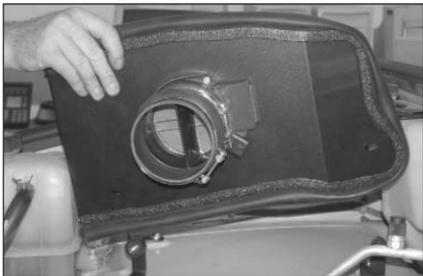
17. Install the heat shield assembly into vehicle as shown.
