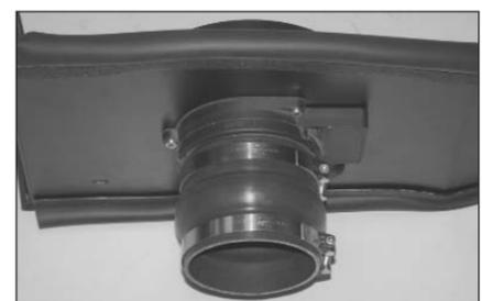
16. Install the silicone hose (084053) onto the K&N intake tube as shown using the supplied hose clamps.
