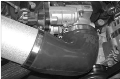
21. Tighten the hose clamp, which secures the silicone hose to the throttle body.
