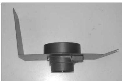
10. Install the mass air sensor and filter adapter onto the heat shield using the gaskets and hardware provided.
