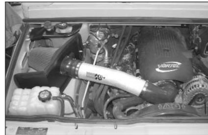
24. Re-install the engine cover removed in step #2 and reconnect the negative battery cable and double check to make sure everything is tightened and properly positioned before starting the vehicle.
