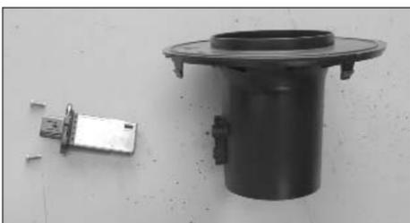
13. On 2006 models, remove the two screws which secure the mass air sensor to the housing and then remove the sensor from the housing as shown.
