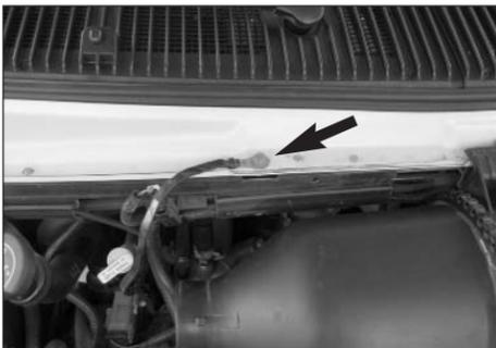
3. Remove the two bolts which secure the air filter assembly to the cowl.
