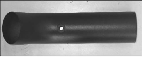
25b. Install the provided grommet into the hole drilled into the intake tube (during the previous step) as shown. Then, install the air temperature sensor into the grommet.
