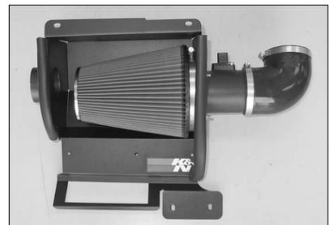
24. Install the K&N filter onto the filter adapter and secure with the provided hose clamp.
