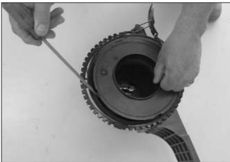
11. Use a screw driver to open the mass air sensor housing and remove the mass air sensor from the housing.
