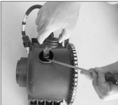
10. Pull back the rubber plug to gain access to the primary mass air sensor connection. Using a small screw driver, release the locking tab and disconnect the mass air sensor electrical connection.
