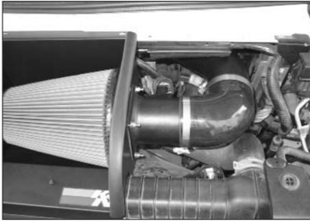
29. Insert the K&N intake tube into the silicone hose at the throttle body and secure with the provided hose clamp.
