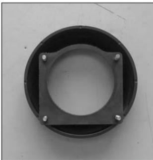
18. Install the mass air gasket to the filter adapter as shown.
