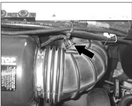
3a. On vehicles equipped with an external air temperature sensor; disconnect the temperature sensor electrical connection.
