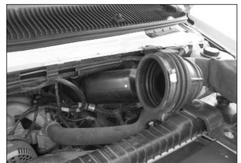
8. Remove the intake tube from the vehicle.
