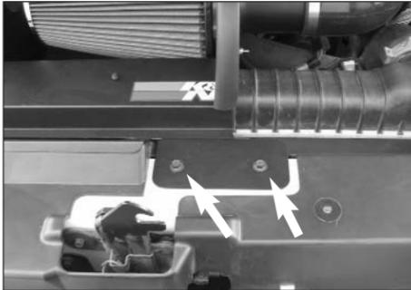
31. Using the factory bolts removed in step #5 secure the heat shield to the radiator core support.
