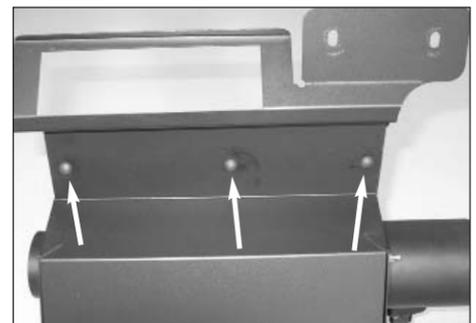
22. Install the three supplied rubber bumpers into the three holes in the heat shield from the bottom up.
