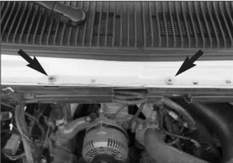
27. Place the two supplied spacers onto the cowl assembly at the air box mounting location as shown.
