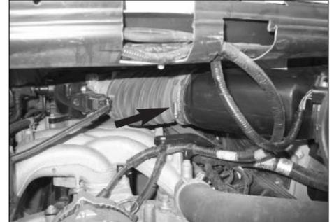
7. Loosen the hose clamp which secures the stock intake tube to the bellows at the throttle body.
