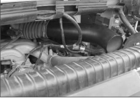
26. Install the K&N intake tube into the bellows at the throttle body and secure with the factory hose clamp.
