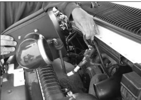
28. Set the filter assembly on top of the radiator assembly, reconnect the mass air sensor secondary connection and then set the filter assembly into position on the cowl and radiator core support.
