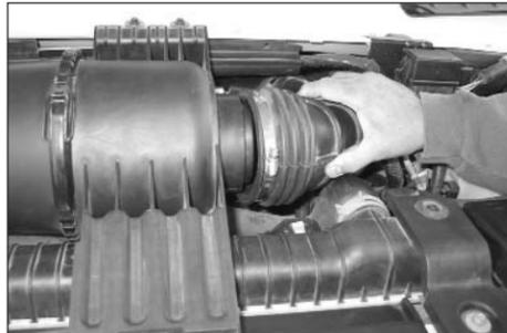
4. Loosen the hose clamp which secures the intake tube to the air filter housing and then disconnect the intake tube from the air filter.
