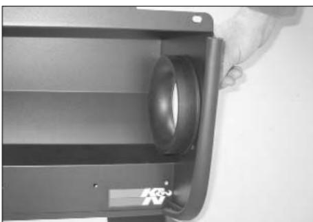
19. Install the filter adapter into the heat shield as shown.
