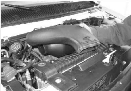
2. Unhook the fresh air intake scoop from the radiator core support and then rotate it back to unlock from the air filter assembly. Then remove it from the vehicle.
