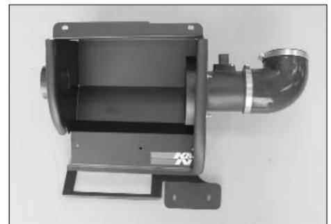
23. Install the silicone hose (084088) onto the mass air sensor housing and secure with the provided hose clamp.
