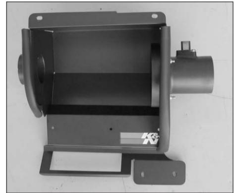
21. Install the mass air sensor assembly onto the studs and secure with the provided nuts and washers.
