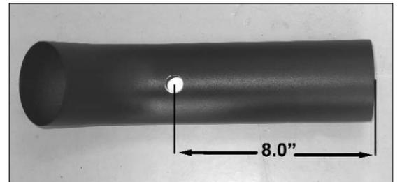
25a. On vehicles equipped with an external temperature sensor; measure and mark the tube 8.0" (from the straight end of the tube, on the inside radius of the bend). Then, drill a 5/8" ID hole in the tube as shown.
