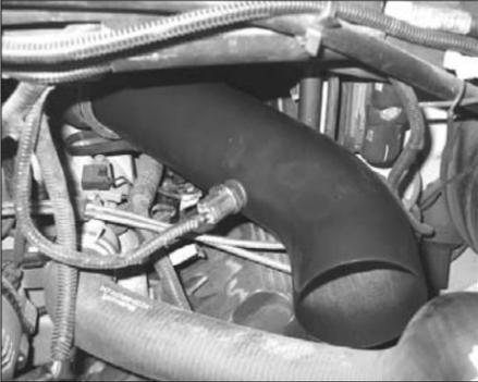
26a. On vehicles equipped with an external air temperature sensor; re-connect the air temperature sensor electrical connection as shown.
