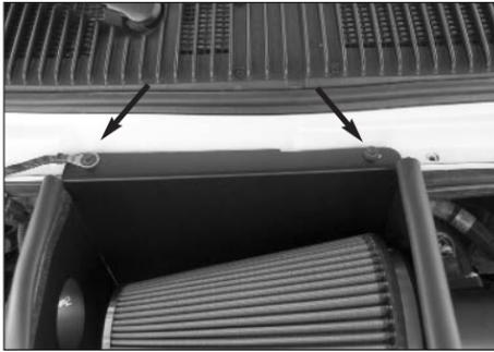
30. Using the factory bolts removed in step #3, secure the heat shield to the cowl.
