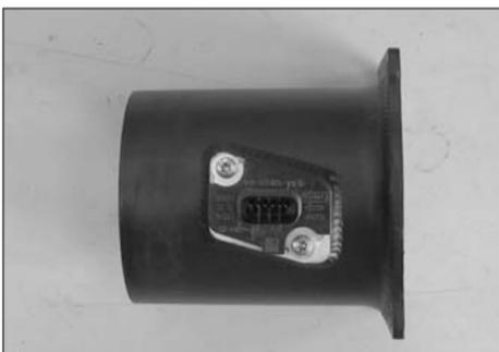
14. On 2006 models, install the mass air sensor removed in step #13 into the K&N mass air sensor housing with the supplied hardware as shown.
