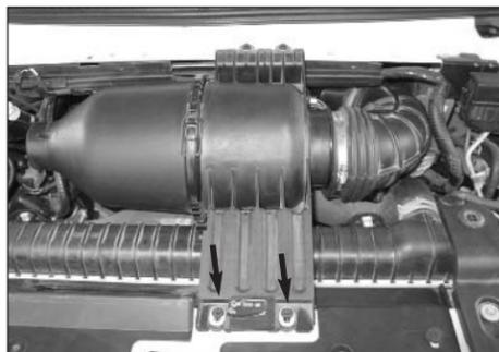
5. Remove the two bolts that secure the air filter housing to the radiator core support.
