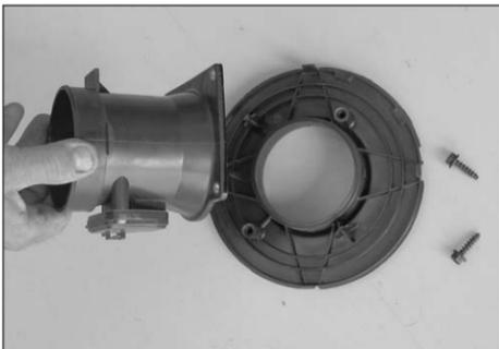
12. On 2005 and earlier vehicles, remove the two bolts that secure the mass air sensor to the mounting plate and then remove the sensor as shown.
