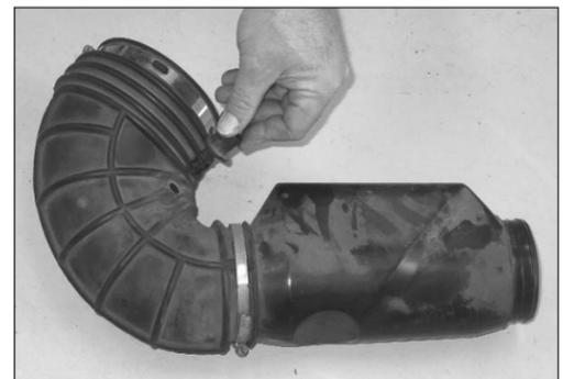
8a. On vehicles equipped with an external air temperature sensor; remove the air temperature sensor from the stock intake tube.
