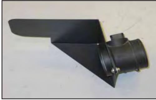
15. Install the mass air sensor onto the heat shield (07352) with the provided hardware as shown.
