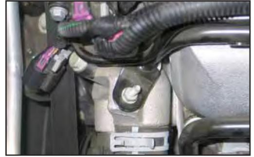
20a. On vehicles equipped with the above style heater hose tube, remove the mounting bolt shown.
