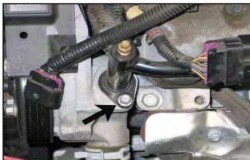
20. On vehicles equipped with the above style heater hose tube, remove the mounting bolt shown.
