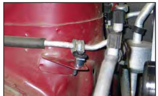
23. With the bolt removed in step #9 and spacer (#07849) secure the A/C line to the inner fender as shown.
