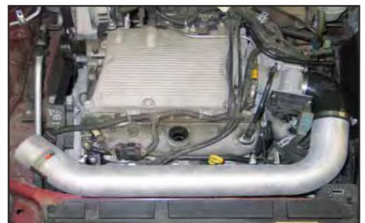
22. Install the K&N Intake Tube into the silicone hose at the throttle body and align the intake tube with the mounting brackets installed in the previous step. Secure the intake tube with the provided hardware and hose clamp.
