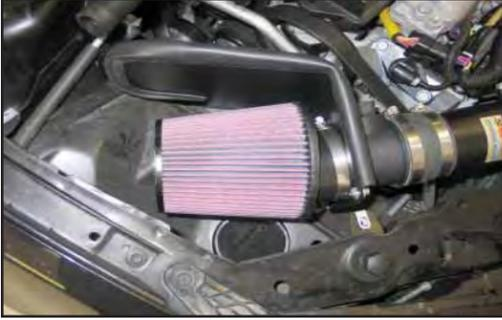
26. Install the K&N Air Filter as shown.
