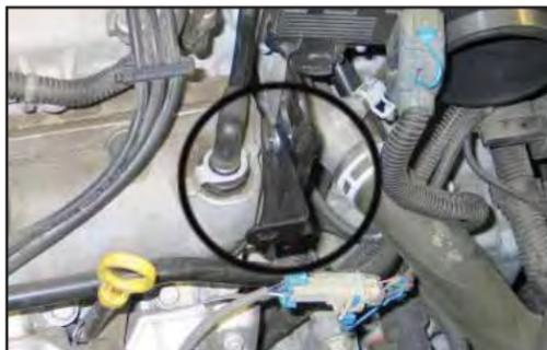
19. Install "L" bracket (#070742) to the 1/4" id hole in the engine lifting bracket using the provided hardware as shown.
