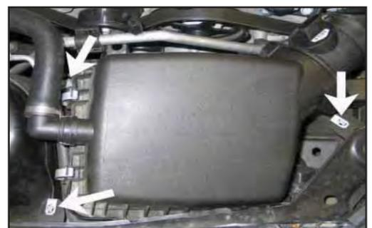
9. Remove the three bolts that secure the stock air box. On vehicles equipped with air injection, release the retaining clips and unhook the air injection hose from the air box lid.
