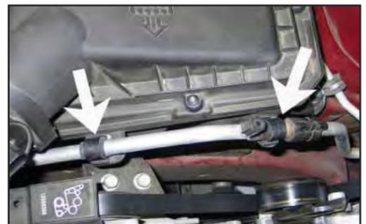
8. Remove the two clamps securing the A/C line to the stock air box.
