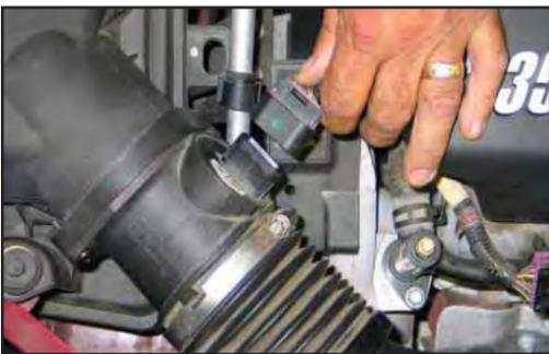
2. Depress the locking tab and disconnect the mass air sensor electrical connection.
