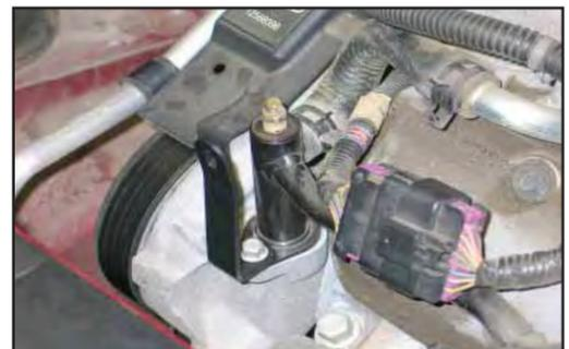
21. Install the correct tube mounting bracket (06496 or 070049) to match the style heater hose tube as shown in the above photos and secure with the factory bolt removed in step #20a.
