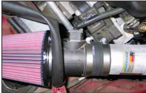
28. Re-connect the mass air sensor as shown.
