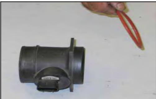
13. Remove the O-ring from the mass air sensor.
