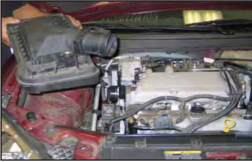
10. Remove the stock air box from the vehicle.
