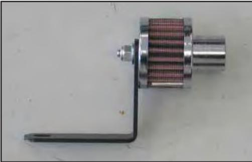
26a. On vehicles equipped with air injection system, secure the provided air injection filter to the mounting bracket (07177) as shown.
