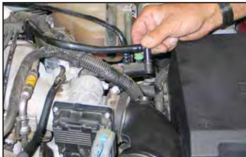
4. Remove the crank case vent tube from the stock intake tube.
