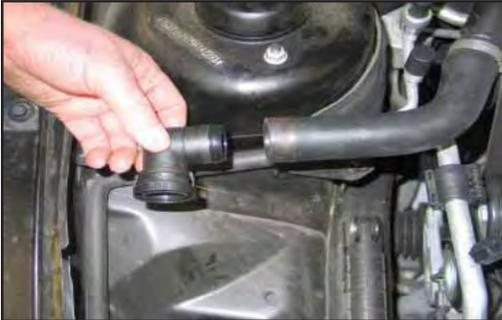
10a. On vehicles equipped with air injection, cut the clamp which secures the elbow fitting to the hose and then remove the elbow fitting from the hose.
