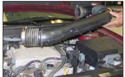
7. Remove the stock intake tube from the vehicle.
