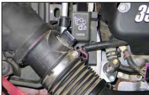
5. Loosen the hose clamp that secures the stock intake to the mass air sensor.
