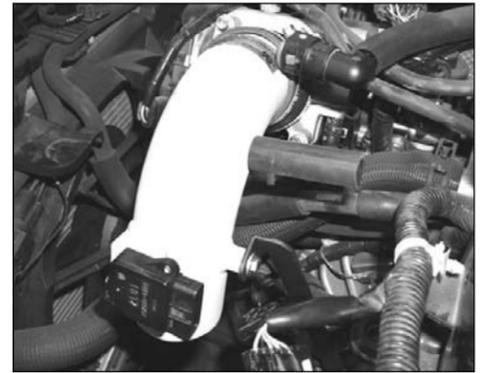
27. Install the K&N intake tube into the silicone hose at the throttle body and align with the mounting bracket. Secure the tube with the provided hardware and hose clamp.
