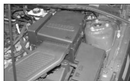
43. Reconnect the negative battery cable, then, reinstall the battery cover as shown.
