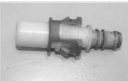
18. Slide the plastic clip from step 15 back onto the crank case vent as shown.
