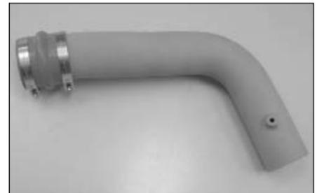
32. Install the silicone hose and hose clamps onto the cold air tube as shown.
