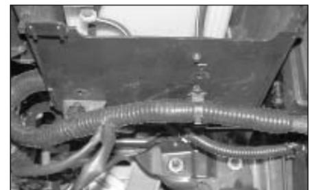
13. Unclip the wire harness from the side of the battery box as shown.
