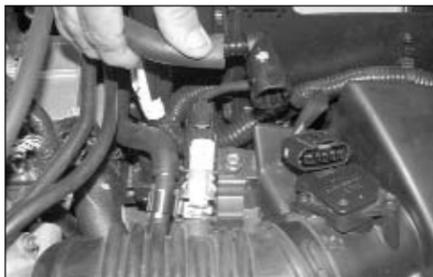
6. Depress the retaining clip and disconnect the crank case vent hose from the stock intake tube as shown.
