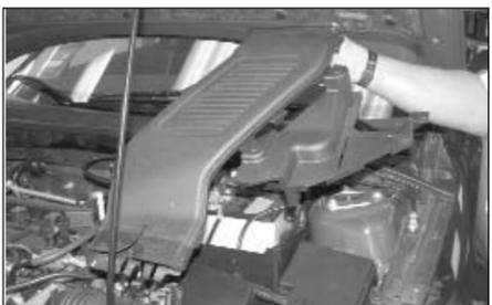
4. Slide the battery cold air vent backwards and remove from the engine compartment as shown.
