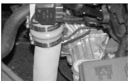
35. Slide the cold air tube onto the short ram tube as shown.
