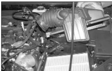
10. Unclip the air cleaner cover and remove the complete upper air cleaner assembly as shown.
