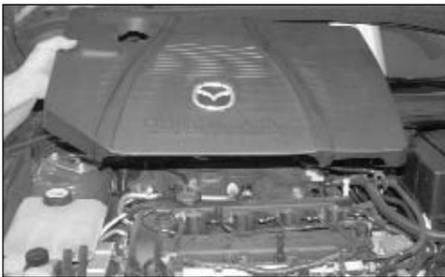
1. Pull firmly upwards to remove the engine cover as shown.
