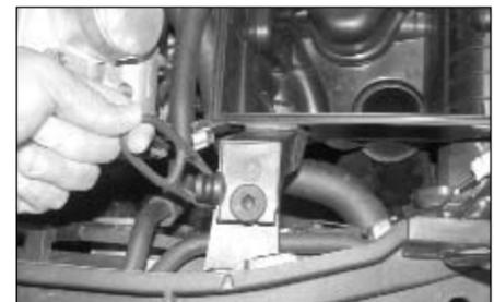
11. Remove the rubber retainer from the core support as shown.
