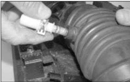
17. Remove the plastic vent from the stock intake tube as shown.
