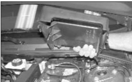
2. Unclip the battery cover and remove, then, disconnect the negative battery cable.
