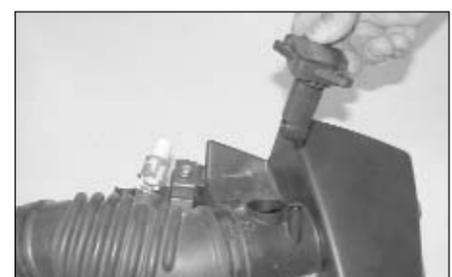
14. Remove the mass air sensor from the air cleaner cover as shown.
