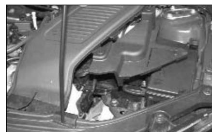
42. Slide the vent into the core support and line up the other end with the battery box and secure with plastic rivet.
