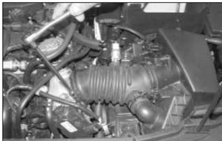
8. Loosen the hose clamp at the throttle body as shown.
