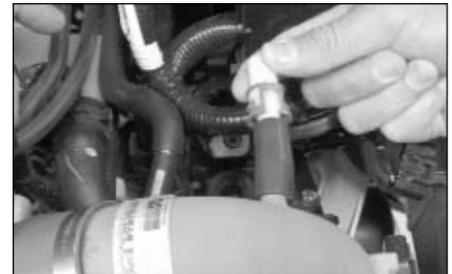
29. Install the crankcase vent from step 18 into the silicone hose on the intake tube as shown.
