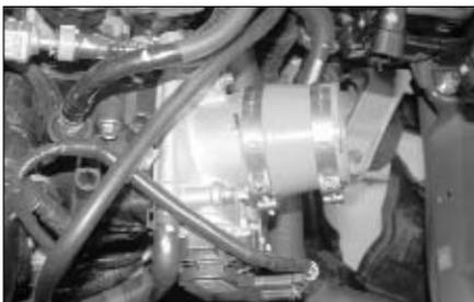
24. Install the silicone hose and hose clamps onto the throttle body as shown.
