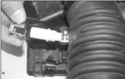
15. Remove the plastic clip from the crank case vent on the stock intake tube as shown.
