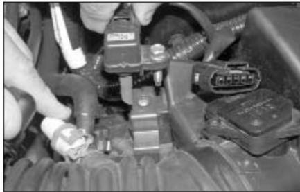
7. Remove the switch/sensor from the air cleaner cover as shown.
