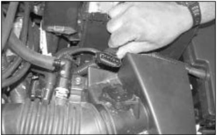
5. Disconnect the mass air sensor electrical connection as shown.
