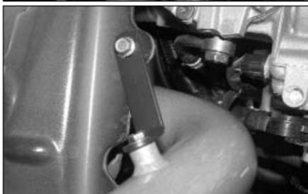
36. Secure the bracket to the rubber mounted stud using the provided hardware as shown.
