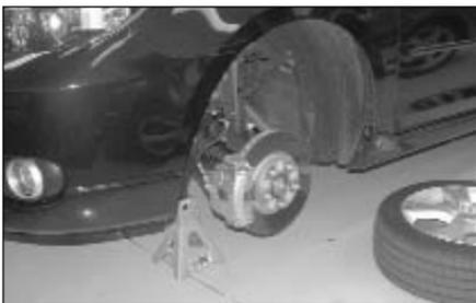
19. Raise the vehicle up and support it with jack stands, then, remove the front tire as shown.
