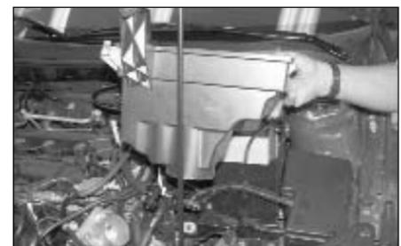
12. Remove the lower air cleaner assembly as shown.
