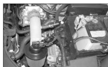
45. This K&N Typhoon kit is designed for use in two different configurations. In the case of inclement weather, the cold air tube can be removed and the filter can be clamped onto the short ram tube located in the engine compartment as shown above, to avoid the possibility of ingesting water into the engine.
