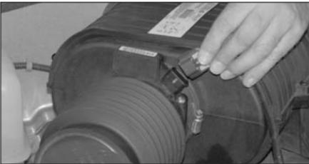
3. Disconnect the mass air sensor electrical connection.
