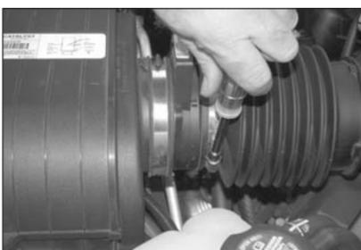
5. Loosen the hose clamp at the mass air sensor.
