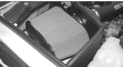
23. Install the air filter onto the mass air sensor and then tighten hose clamp.
