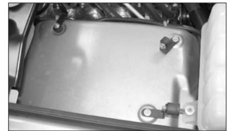
15. Install the 3 brackets onto the vehicle with the provided hardware as shown. Don't tighten completely at this time.
