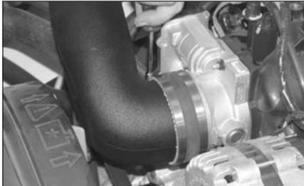
22. Align the intake tube with the throttle body then tighten the hose clamps.
