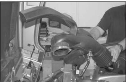
6. Detach the intake tube from the throttle body and mass air sensor then remove the intake assembly.
