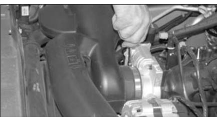
4. Loosen the hose clamp at the throttle body.
