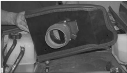
18. Install the heat shield assembly into vehicle as shown.
