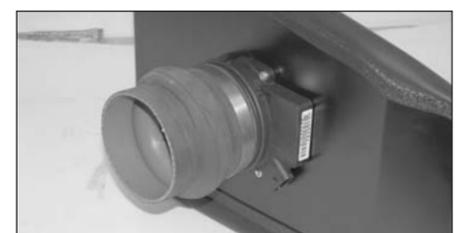
16. Install the silicone hump hose (08176) onto the mass air sensor with the provided hose clamps as shown.
