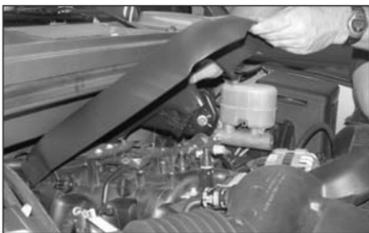
2. Remove the 8mm bolt that retains the engine cover onto the engine then remove the cover from vehicle.
