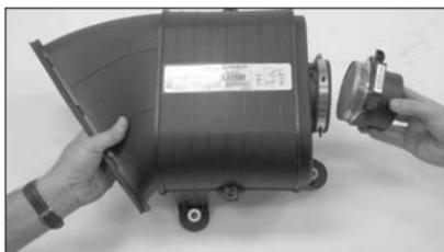
9. Loosen the hose clamp that retains the mass air sensor onto the air box then remove the mass air sensor from the air box.
