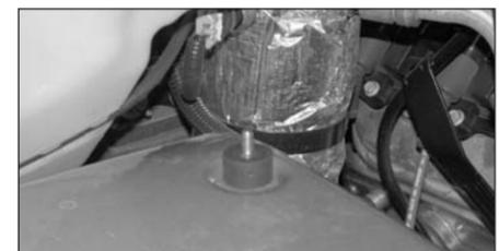
14. Install the rubber mounted stud onto the vehicle as shown.
