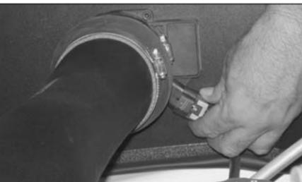
24. Reconnect the mass air electrical connection as shown.
