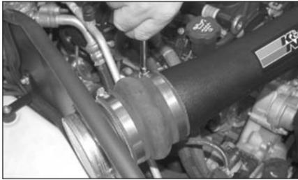
21. Install the intake tube onto the vehicle then align the tube with the mass air sensor and then tighten hose clamp.
