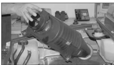
8. Remove the air box from vehicle as shown. NOTE: K&N recommends that customers do not discard factory air intake.
