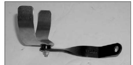
13. Install saddle bracket onto new bracket as shown.
