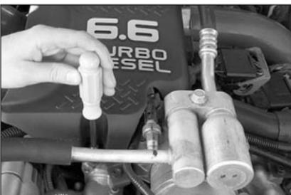
3. On 2001 models, remove the 8mm bolt that retains the engine cover, then remove cover.
