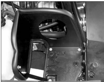
11. Mount the heat shield onto the airbox mounting tray and secure with the three bolts removed in step 10.
