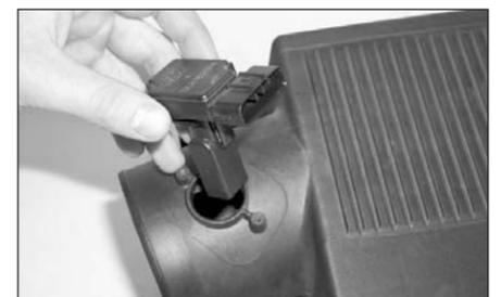
15. Loosen and remove the two torx screws that retain the mass air sensor with the provided torx wrench, then remove sensor.
