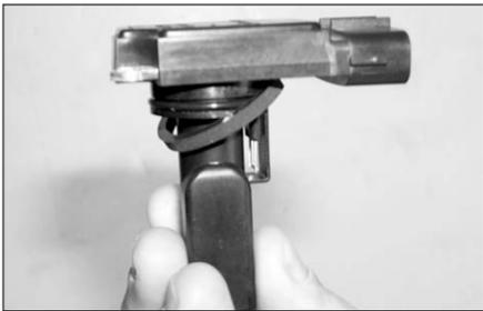
17. Install new gasket onto mass air sensor as shown with sticky side towards mass air sensor.
