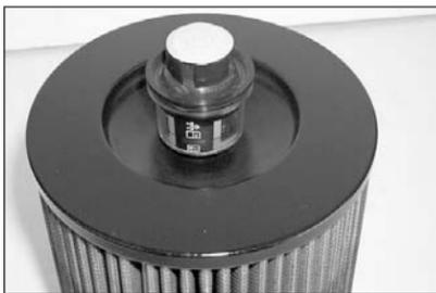
24. Install filter restriction gauge onto filtercharger as shown.
