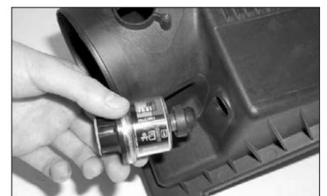
16. Remove the restriction gauge and grommet from the stock airbox assembly as shown.
