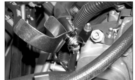
14. Secure bracket onto stud and secure bracket with nut that was removed in step 12. Do not tighten completely.
