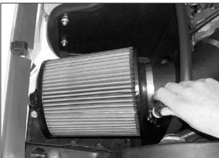
25. Install the K&N filtercharger onto intake tube as shown then tighten completely.
