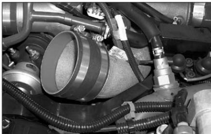
19. Install silicone hose onto intake manifold with provided hose clamps.
