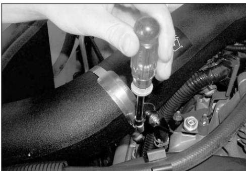
21. Install saddle bracket onto intake tube with hose clamp provided. Adjust for best fit and tighten all hardware.
