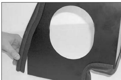
8. Apply the provided trim seal to the heat shield assembly as show. Trim if necessary.
