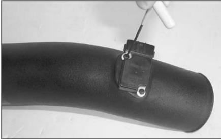
18. Install spacers under mass air sensor then attach mass air sensor onto new K&N intake tube with hardware provided.
