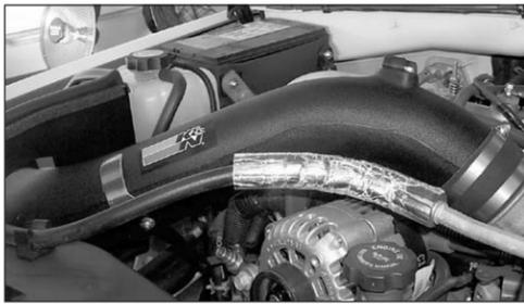
20. Secure the K&N intake tube to the intake manifold with the provided hose clamp.
