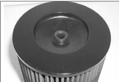
23. Install grommet onto filter as shown.
