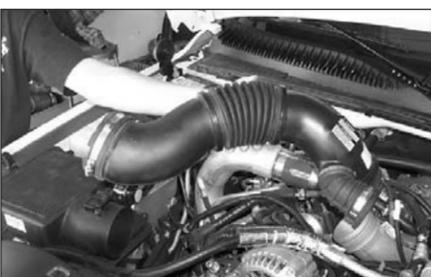
6. Loosen hose clamp at intake manifold and airbox, then remove complete air intake tube.
