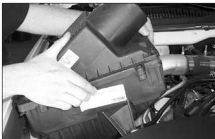
7. Pull firmly upwards on stock airbox to remove from vehicle.
