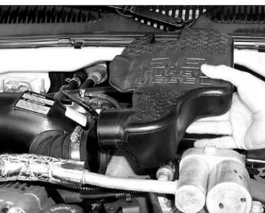
5. Loosen hose clamp at intake resonator then remove resonator from vehicle.
