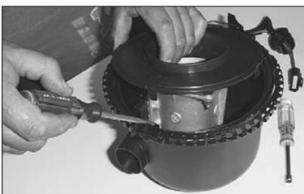
10. Using a flat blade screwdriver, push in and release the four clips that retain the mass air sensor retaining plate.
