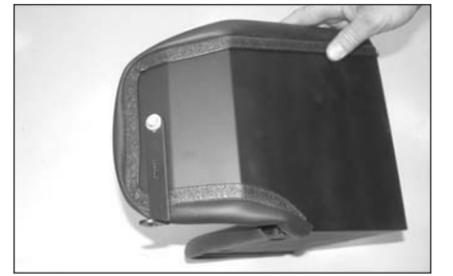
15. Install the provided "L" bracket (070952) onto heat shield as shown. NOTE: Install a washer between heat shield and bracket.
