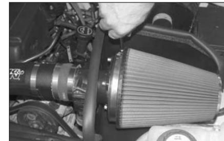
31. Install the Filtercharger onto the mass air sensor and secure it with the provided hose clamp.
