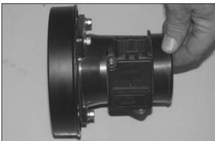
24. Attach the mass air adaptor to the mass air sensor using the gasket and provided hardware as shown.
