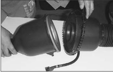
8. Open the air cleaner assembly and isolate the mass air sensor assembly.
