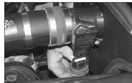
30. Reconnect the primary and secondary mass air electrical connection.
