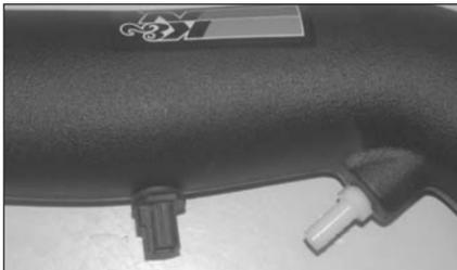
23. Install the temp sensor into the new K&N intake tube as shown.
