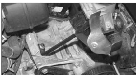
19a. On non A/C vehicles, install the saddle bracket assembly from step 18 onto vehicle with the provided hardware as shown.
