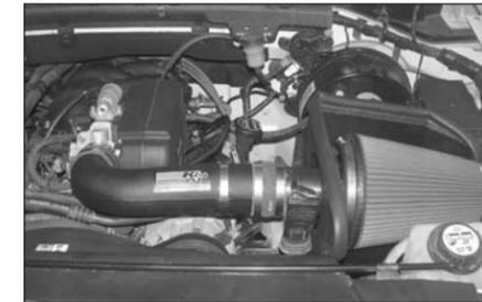
32. It may be necessary to loosen clamps and twist the entire assembly to achieve proper alignment and clearance, then re-tighten all hardware.
