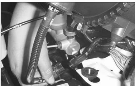
6. Disconnect the secondary mass air sensor electrical connection.
