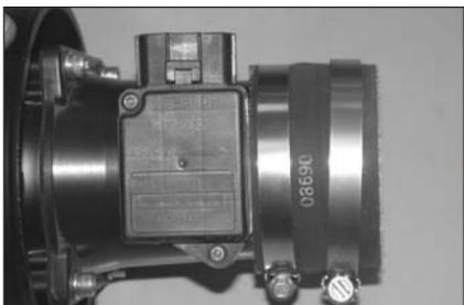
25. Install the silicone hose (08690) onto the mass air assembly with the provided hose clamps as shown.
