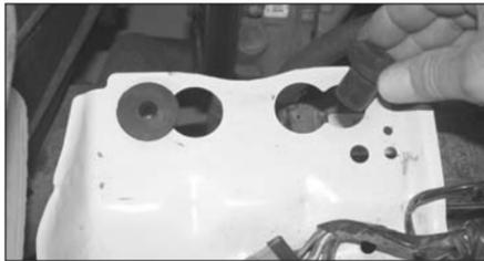
16. Install the two nut inserts onto the air box mounting tray as shown.
