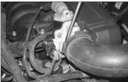
4. Loosen hose clamp at the throttle body.
