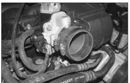
20. Install the provided silicone hose (08756) onto the throttle body with the provided hose clamps.
