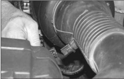
2. Disconnect the air temp sensor electrical connection.
