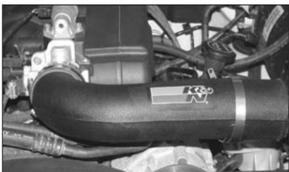
26. Install the K&N intake tube onto the throttle body, then align with the saddle bracket. Then tighten all hose clamps.
