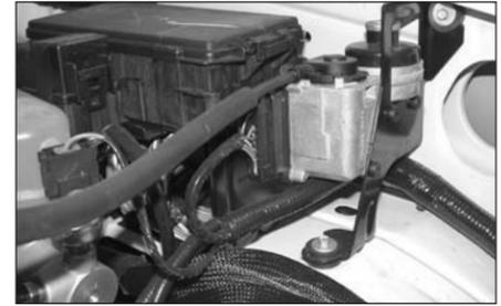
14. Remove the 6mm bolt that retains the cruise control onto vehicle.
