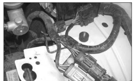
14a. On vehicles without cruise control, install the rubber mounted stud onto vehicle as shown.
