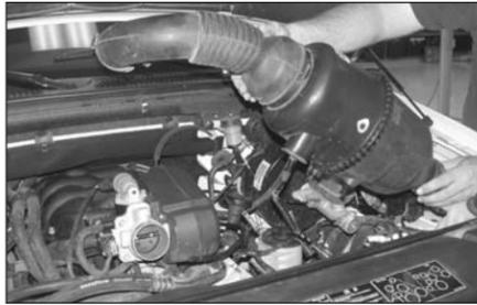
7. Remove the entire stock air intake assembly from the vehicle.
