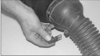
21. Remove the temp sensor from the stock intake tube as shown.
