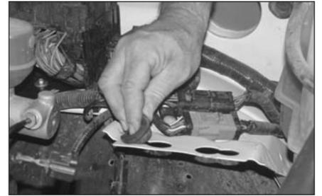
12. Remove the two air box mounting grommets from vehicle as shown.
