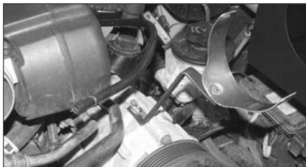
19. On vehicles that come equipped with A/C, remove the A/C mounting bolt. Then secure saddle bracket assembly from step 18a onto vehicle with the bolt that was removed.
