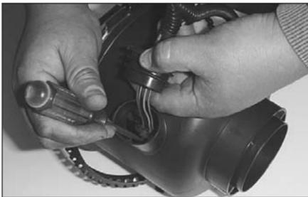
9. Slide the rubber grommet back and disconnect the primary mass air sensor electrical connection, using a flat blade screwdriver.
