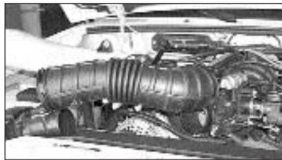
6. Loosen the hose clamp at the throttle body and at the mass air sensor, then remove the stock air intake tube as shown.
