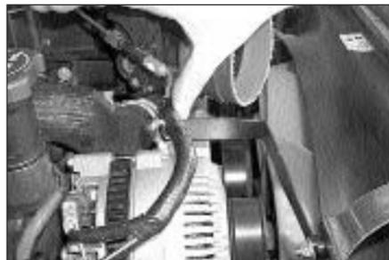
15. Push the wire harness push clip into the hole on the saddle bracket as shown.
