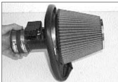
22. Assemble the K&N Air filter onto the heat shield assembly as shown.
