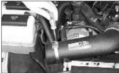
19. Re-install the K&N intake tube onto the throttle body then secure the intake tube to the saddle bracket assembly with the provided hose clamp.
