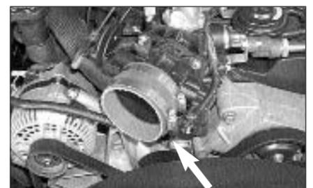
12. Install the silicone hose (08630) and the hose clamps onto the throttle body as shown.
