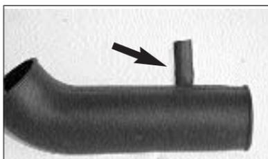
16. Install the rubber hose onto the K&N intake tube as shown.
