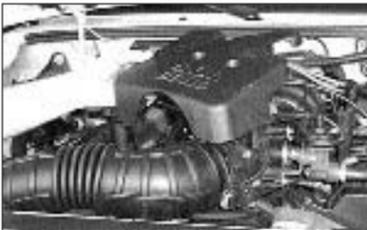
3. Loosen and remove the three bolts that secure the throttle body cover, then remove the cover as shown.
