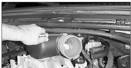
24. Install the stepped hose onto the throttle body and tighten hose clamp.
