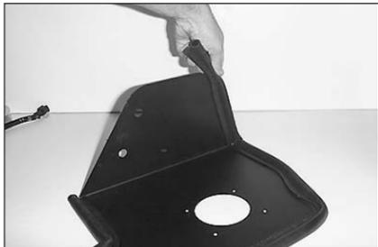
19. Install the trim seal onto the heat shield as shown.
