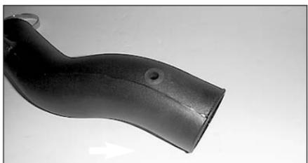
23. On models equipped with an external air temperature sensor, insert the grommet into the hole drilled in the K&N intake tube.
