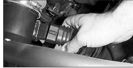
33. Reconnect the primary mass air sensor electrical connection.
