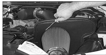
37. Install the Filtercharger element and tighten hose clamp.
