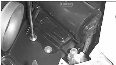
29. Position the heat shield for best alignment and tighten the hardware that retains it.
