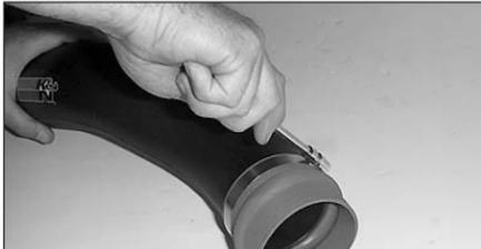
25. Install the hump hose onto the intake tube and tighten hose clamp.
