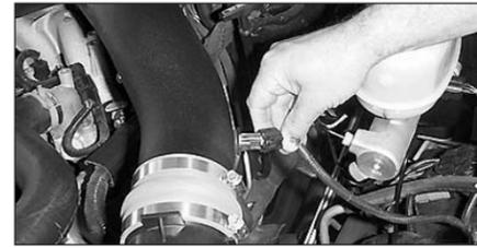
36. On models equipped with an external air temperature sensor, reconnect the air temperature sensor electrical connection and relocate the wiring harness retaining clip to front hole in the inner fender apron.
