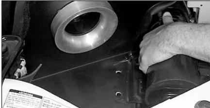
26. Lift up on the evaporative canister mounting bracket and install the heat shield.
