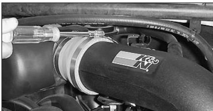
28. Position the intake tube for best alignment and tighten the hose clamp on the stepped hose at the intake tube.
