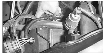
34. Reconnect the secondary mass air sensor electrical connection and reattach the wiring harness retaining clip to the inner fender apron.
