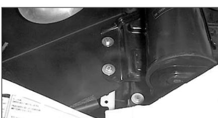
27. Install the hardware to retain the heat shield.
