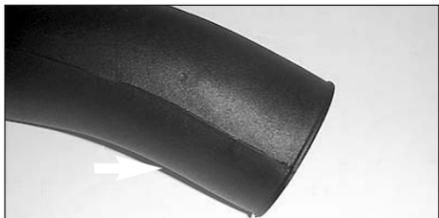
22. On models equipped with an external air temperature sensor, drill out the drill point in the K&N intake tube using a 11/16" drill bit.
