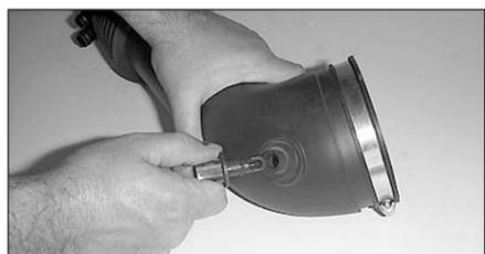
21. On models equipped with an external air temperature sensor, remove the air temperature sensor from the stock intake tube.
