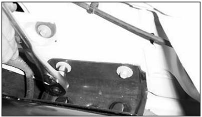
30. Tighten the two bolts that retain the evaporative canister mounting bracket to the inner fender.
