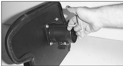
20. Assemble mass air sensor, heat shield and adapter using the gaskets and hardware provided.
