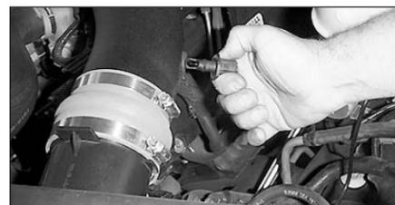
35. On models equipped with an external air temperature sensor, insert the air temperature sensor into the grommet in the intake tube.
