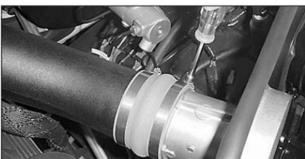
31. Tighten the hose clamp on the hump hose at the mass air sensor.
