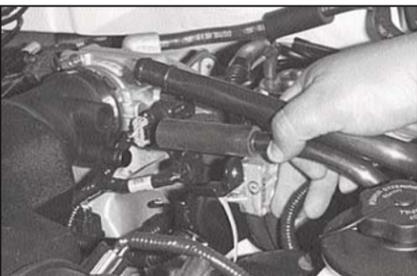
4b. On models with 5.4L, detach the idle air control and crankcase vent hose from the stock intake tube.
