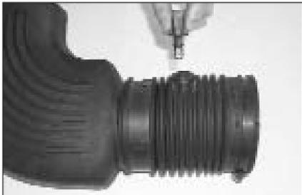
14. Remove the air temp. sensor from stock air intake tube as shown.
