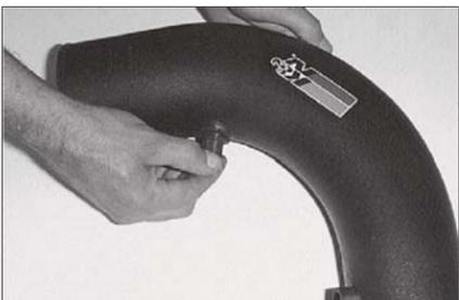
15. Using the grommet provided, install the air temperature sensor into the K&N intake tube.
