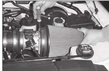
26. Install the Air filter element onto the mass air adapter and secure it with hose clamp provided.
