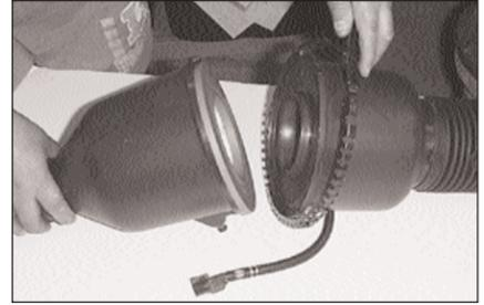
9. Open the air cleaner assembly and isolate the mass air sensor assembly.
