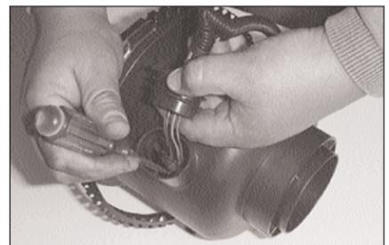
10. Slide the rubber grommet back and disconnect the primary mass air sensor electrical connection, using a flat blade screwdriver.
