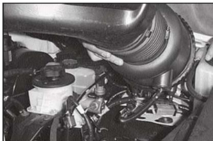
6. Detach the stock intake tube from the throttle body and lift up on the air cleaner assembly to release it from its retaining grommet.
