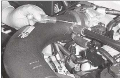
20a. On models with 5.4L engines, install the idle air control and crankcase vent hose onto the appropriate fittings on the K&N intake tube, secure with the hose clamps provided.
