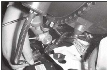
7. Disconnect the secondary mass air sensor electrical connection.
