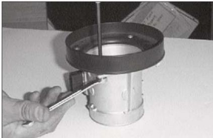
13. Attach the mass air adapter to the mass air sensor using the gasket and hardware provided as shown above.
