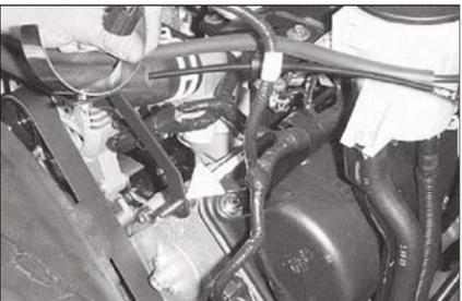
17. Install the saddle bracket assembly onto the protruding stud as shown, secure into place using the hardware provided.
