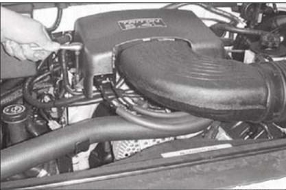
2. Loosen and remove the three bolts that retain the throttle body cover, then remove the cover.
