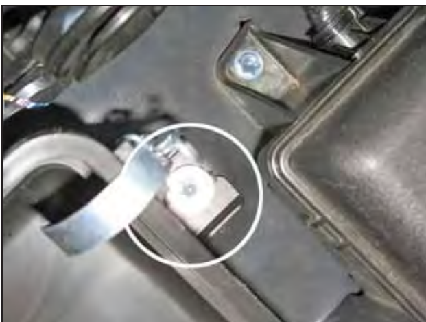
m. Remove the second bolt securing the lower airbox.
