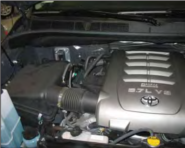
a. Factory airbox system installed.
