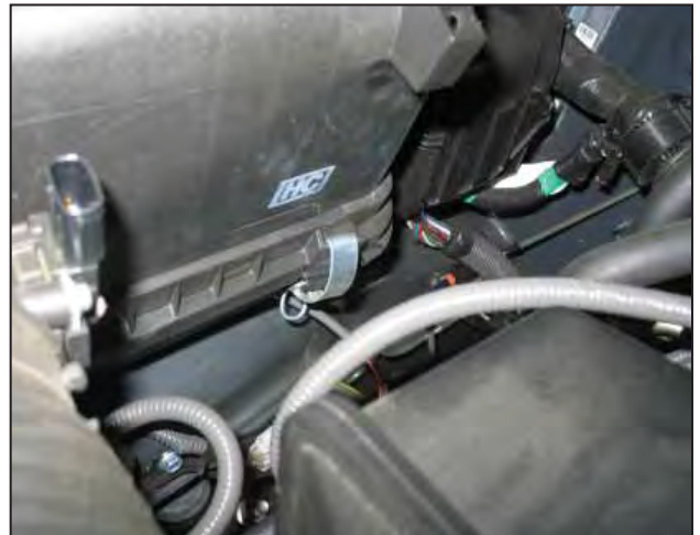
h. Unclip the fourth airbox clip.
