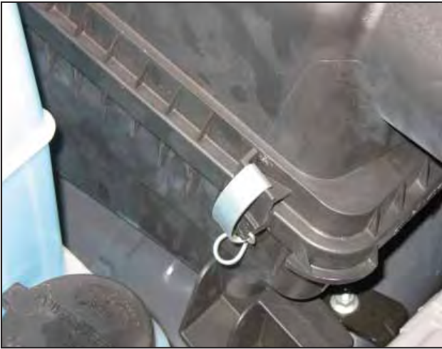
e. Unclip the four clips securing the airbox lid to the lower airbox. This is the first clip.
