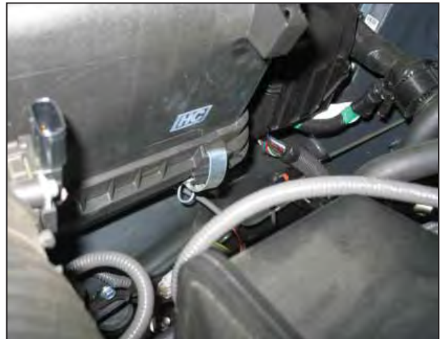
h. Unclip the fourth airbox clip.
