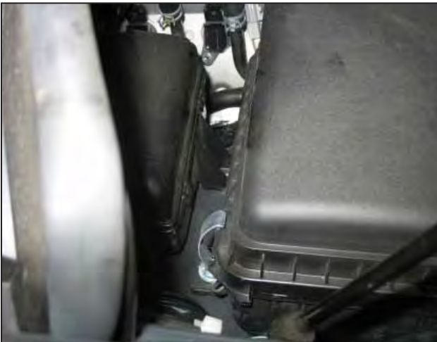
g . Unclip the third airbox clip.
