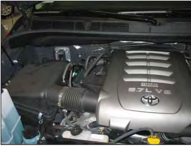
Factory airbox system installed
