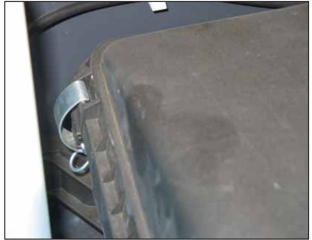
f. Unclip the second airbox clip.
