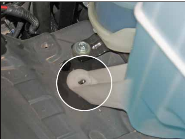
o. Remove the bolt securing the windshield washer fluid container.
