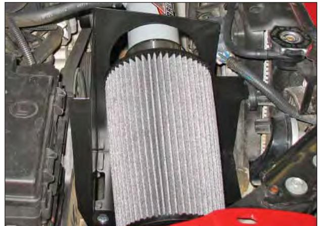
m. Install the AEM® air filter onto the intake tube and secure in place with the supplied #52 hose clamp.
