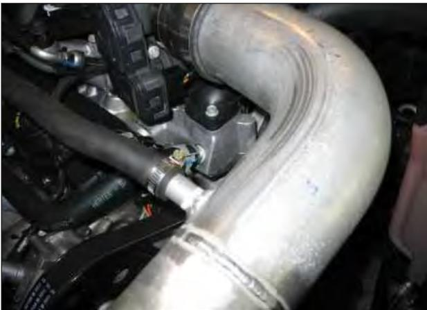
l. Attach the stock breather hose to the intake pipe nipple, secure with the supplied hose clamp.
