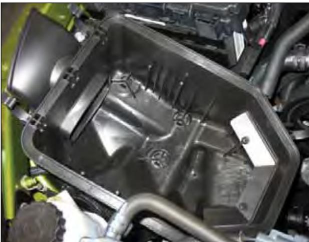
g. Remove the stock air filter and remove the lower airbox by pulling straight up.
