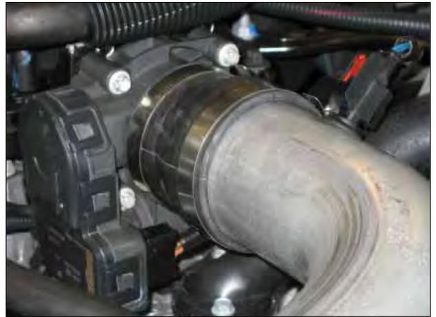
i. Slide the intake pipe into the coupler and loosely secure with the provided hose clamps (#44 hose clamp on the throttle body and a #52 hose clamp on the intake pipe side).
