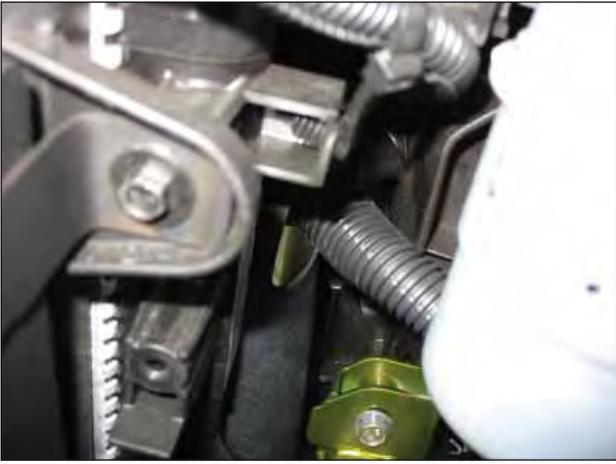
f. Secure the heat shield's tab to the fan shroud using the stock screw removed in step 2i.
