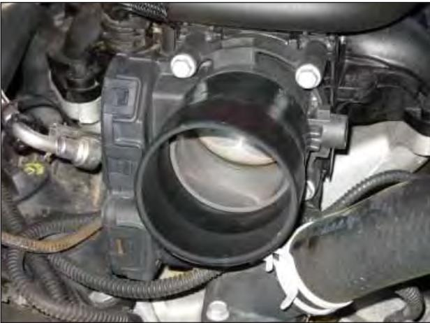
h. Attach the coupler onto the throttle body.
