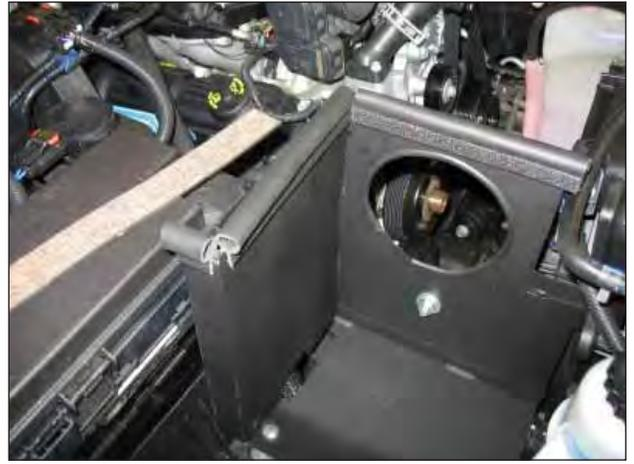
g. Secure the rubber mount to the heat shield with the supplied washer and nut. Install the edge trim onto the heat shield's top edge, also line the heat shield's opening with the supplied rubber edge trim.
