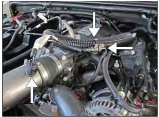
k. Install the grommet into the intake pipe's small inlet hole, then insert the IAT sensor into the grommet. Connect the IAT extension harness to the factory IAT harness and then connect the extension harness connector to the IAT sensor. Secure the wire harness with the supplied zip tie so it is situated in a safe position as shown.
