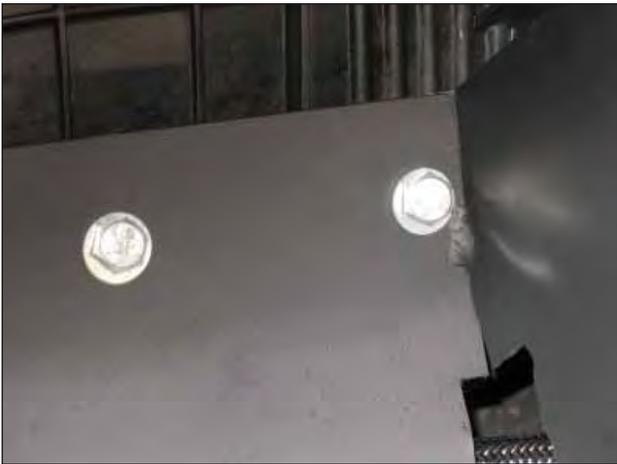
d. Insert the hardware assembled in step 3b through the heat shield holes. Guide the bolts through the spacers that were installed in the previous step.
