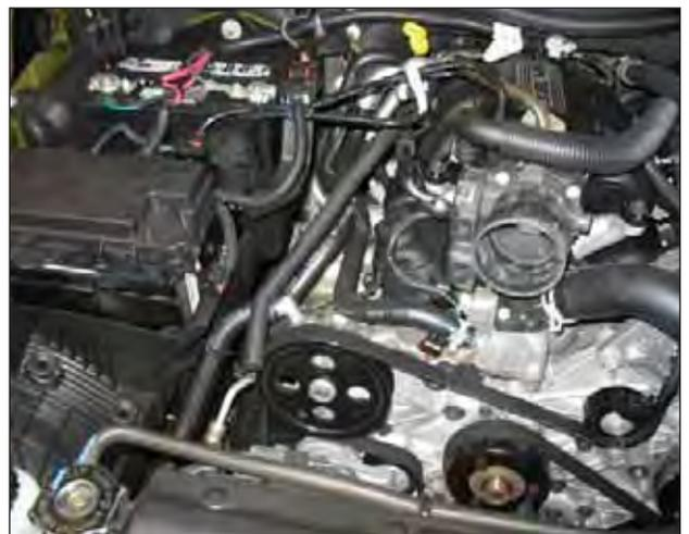
j. Engine bay after the stock airbox system has been removed.
