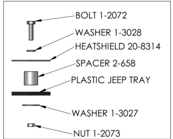
e. Secure the bolts with the supplied washers and nuts to secure the heat shield. Refer to the diagram for proper assembly.
