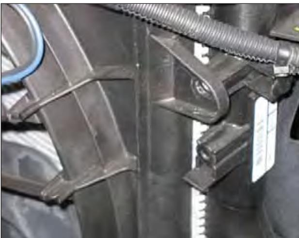
i. Remove the self tapping screw securing the fan shroud. Keep this screw for later use.
