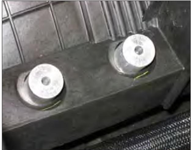
c. Place the two supplied spacers into the inserts that the lower stock grommets were removed from during step 2h.
