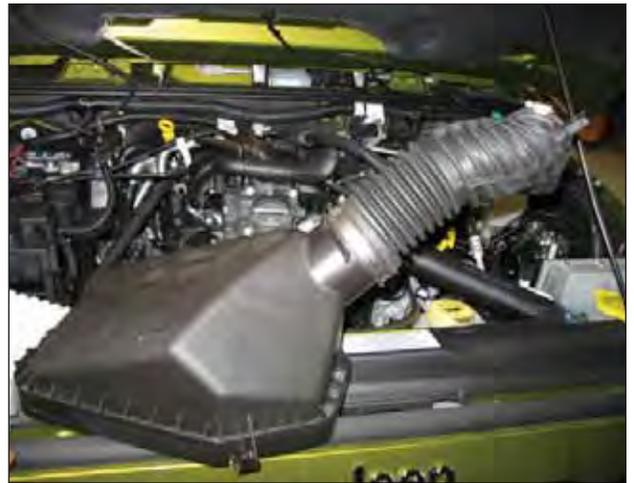
f. Slide the inlet tube off the throttle body and remove the inlet tube and air filter lid as an assembly. Remove the IAT sensor from the inlet tube and set aside in a safe area.
