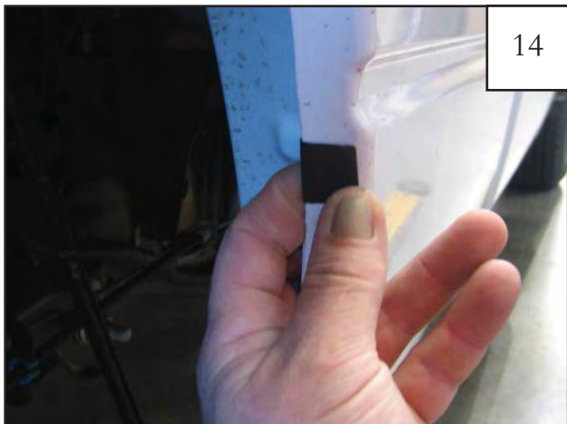
Wrap a black tab around the wheel well sheet metal, centered over each of the four marks made in Step 13.
