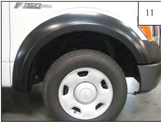
Completed front flare installation.
