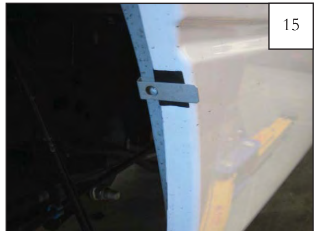
Install a long clip over each of the four black tabs placed on the sheet metal in Step 14.
