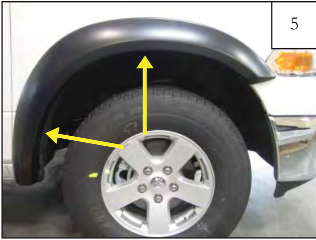
Hold flare to vehicle and start the kit supplied #8 pan-head screws with a Phillips screwdriver. Do not tighten.
