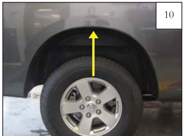
Install speed clip in this location. See step 11.
