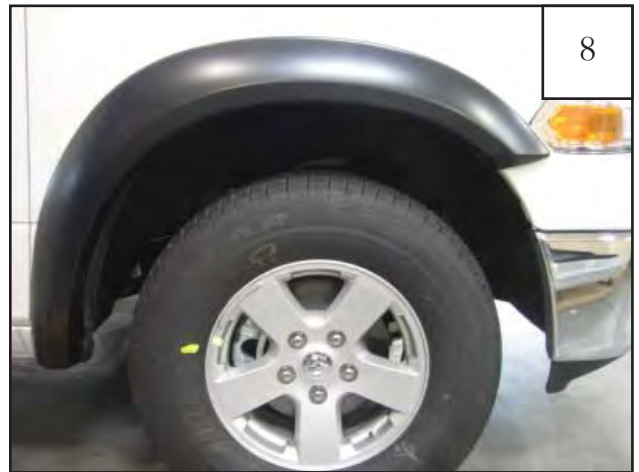
Completed front flare installation.
