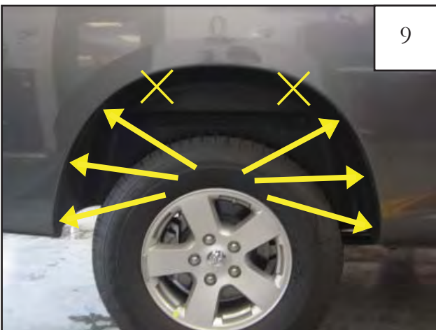
Remove six factory installed screws using an 8 mm socket wrench. Keep screws for installation of the rear flare. X's indicate a factory screw that will not be removed.
