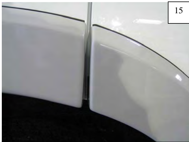
Position Rear Main Flare on fender, aligning with edge of sheet metal along door, but not extending into the door seam.
