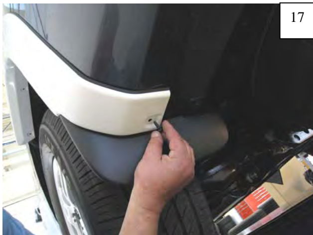
Hand start a supplied Hex bolt in underside of Rear Main Flare at mud flap area. Do not tighten.
