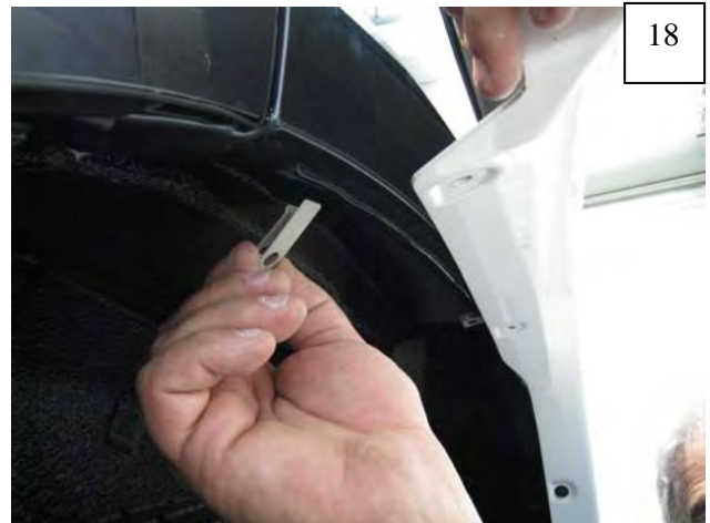
Pull forward portion of flare out from fender gently, and slide two supplied Long Clips onto fender lip, aligning holes in clips with holes in flare.
