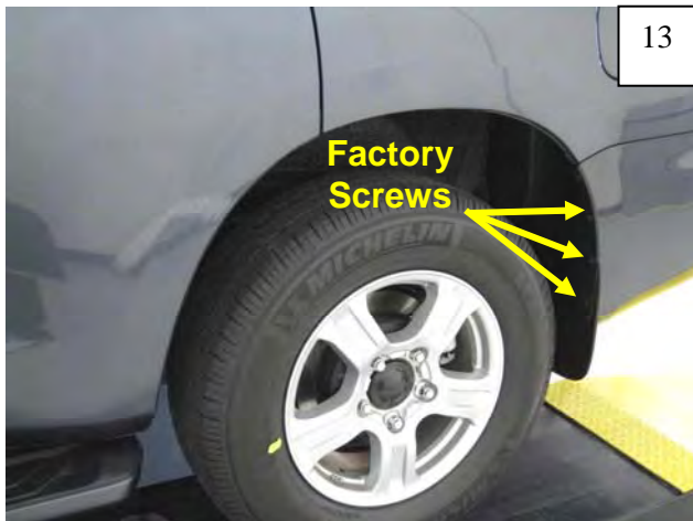
Remove top three screws from rear of rear wheel well. Discard
