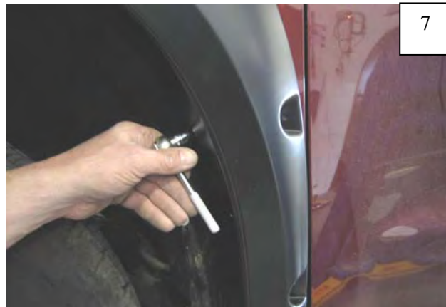
Start a supplied Hex Screw through top rear hole in flare and into factory hole in rear of wheel well. Do not tighten.
