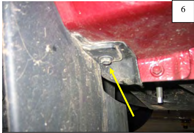
Remove one hex bolt from underside of mud flap. Discard mud flap.
