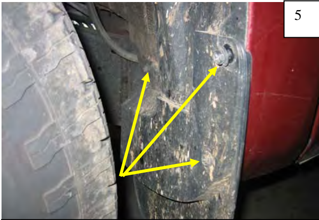
Remove three hex bolts from factory mud flap, using a 10mm socket.
