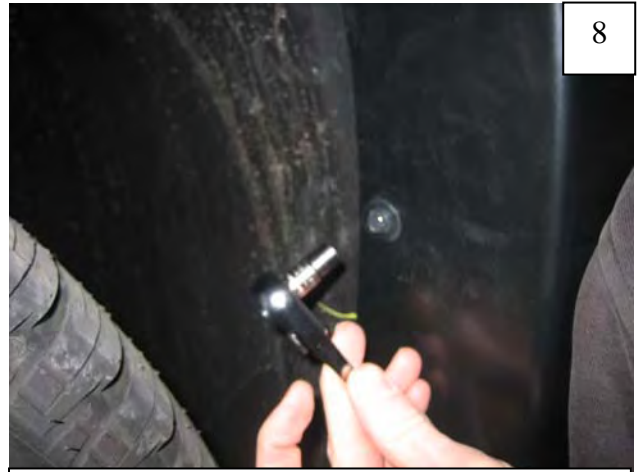
Holding flare in position on fender, reinstall factory screws removed in Step 5.
