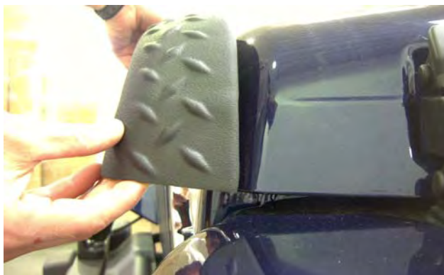
Photo #5 – Hood Protector placement
