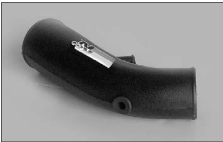
15. Install the grommet into the new intake tube.
