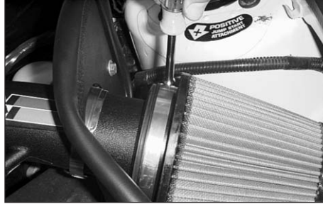
21. Install the air filter onto the intake tube.
