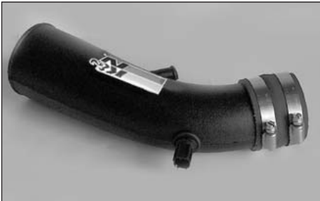
17. Install the silicone hose and hose clamps onto the new intake tube.
