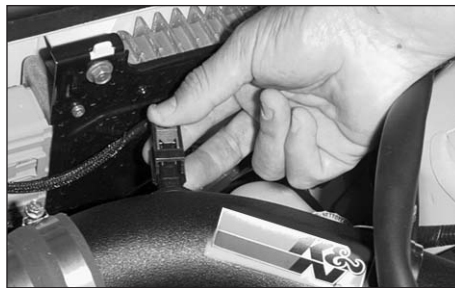
23. Reconnect the air temperature sensor electrical connection.
