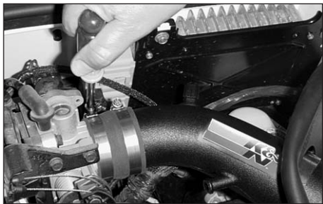
18. Install the air intake tube onto the throttle body.
