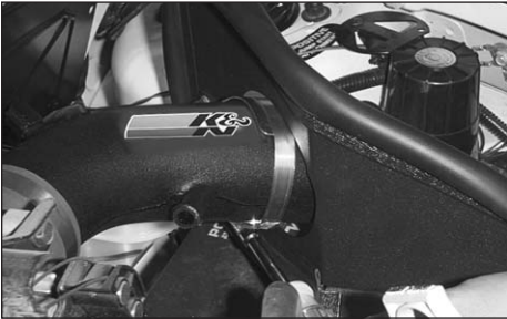
19. Secure the intake tube to the saddle bracket with the hardware provided.
