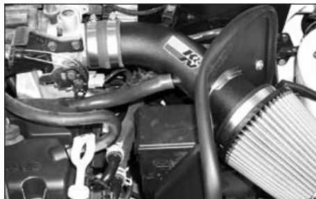
22. Install the crank case vent hose onto the intake tube and valve cover.
